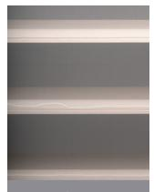
Worm tracks may appear as a slight crease that travels horizontally near the front of the vane, typically seen on the face sheer and in light-dimming fabrics.
